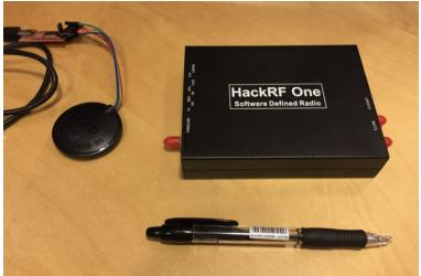
€10 GNSS receiver €250 software based radio that can be used to manipulate the receiver
